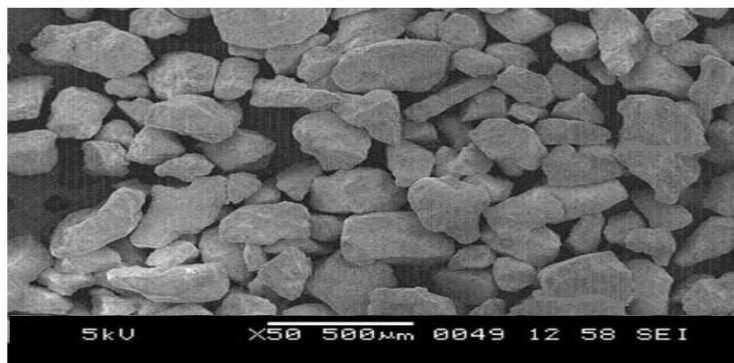
Figure 2(b): SEM Picture of Silica Sand (200-250 \mu\text{m} )
