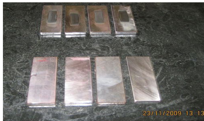
Figure 1. Standard test specimen of size 75mmX 26mmX6mm
